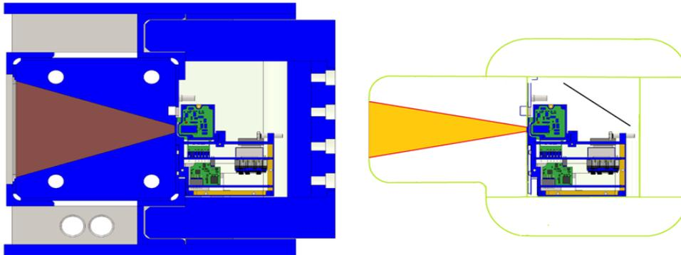
Figure 1 Side view of existing collimator (left). The blue regions represent tungsten. On the right is a concept for a smaller collimator that includes reducing the collimator opening angle and the internal volume for the electronics.
